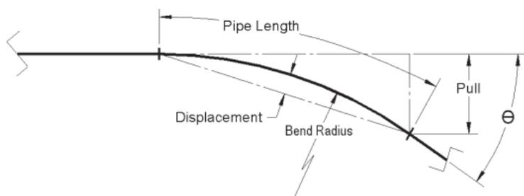
Figure 1. Bend Radius of Pipe
