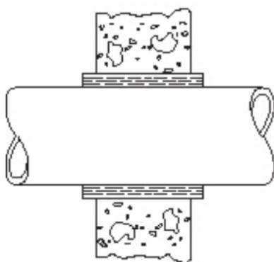
Figure 5. Wall penetration
