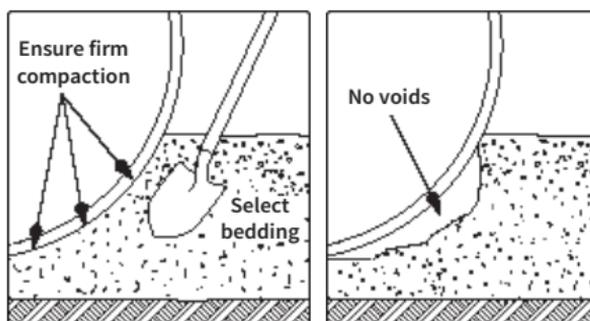
Figure 4. Proper Haunch Filling
