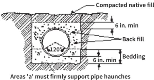
Figure 3. Proper bedding & backfilling
