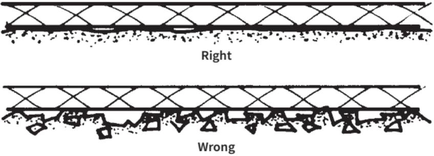
Figure 2. Proper trench bottom preparation
