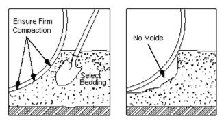
small stones or debris into the pipe wall if they are present in the bedding material. Avoid striking the pipe with tamping equipment as the pipe may be fractured.
