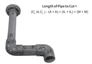
\*CAUTION: Make-up dimensions depend on the tightness of the dry fit. If the field developed dimensions vary, use field developed dimensions.
