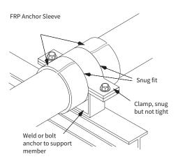
connections. Provisions for expansion should be designed into each of the individual pipe sections.
