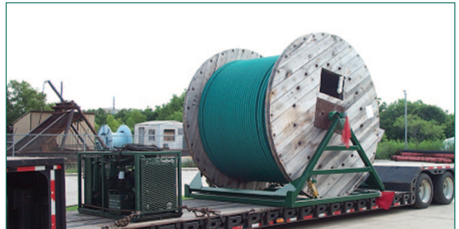
A-Frame Deployment System. Designed for installing 3 1/2" nominal LinePipe and smaller diameters for new construction and pipeline remediation. Two deployment systems can be loaded on a single double-drop flatbed trailer. Equipped with 13-hp hydraulic power unit.
