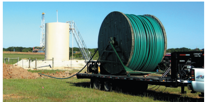
Single Line Deployment System. Gooseneck trailer-mounted deployment system for single lines or smaller diameter applications. Can be brought to location by a Fiberspar service technician with 1 ton, dually-type service vehicle. Equipped with 10-hp hydraulic power unit.
