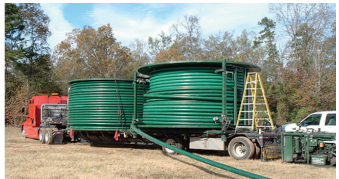
Horizontal Carousel Deployment System. Designed for installing larger diameter Fiberspar LinePipe in standard 4", 4 1/2" and 6 1/2" nominal diameters on 16-ft reels. Carousels also can accommodate non-standard LinePipe. Carousels are normally used on flatbed trailers. Equipped with 24-hp hydraulic power unit.
