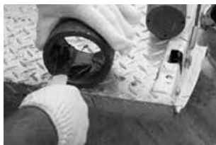
Apply paste to mold
